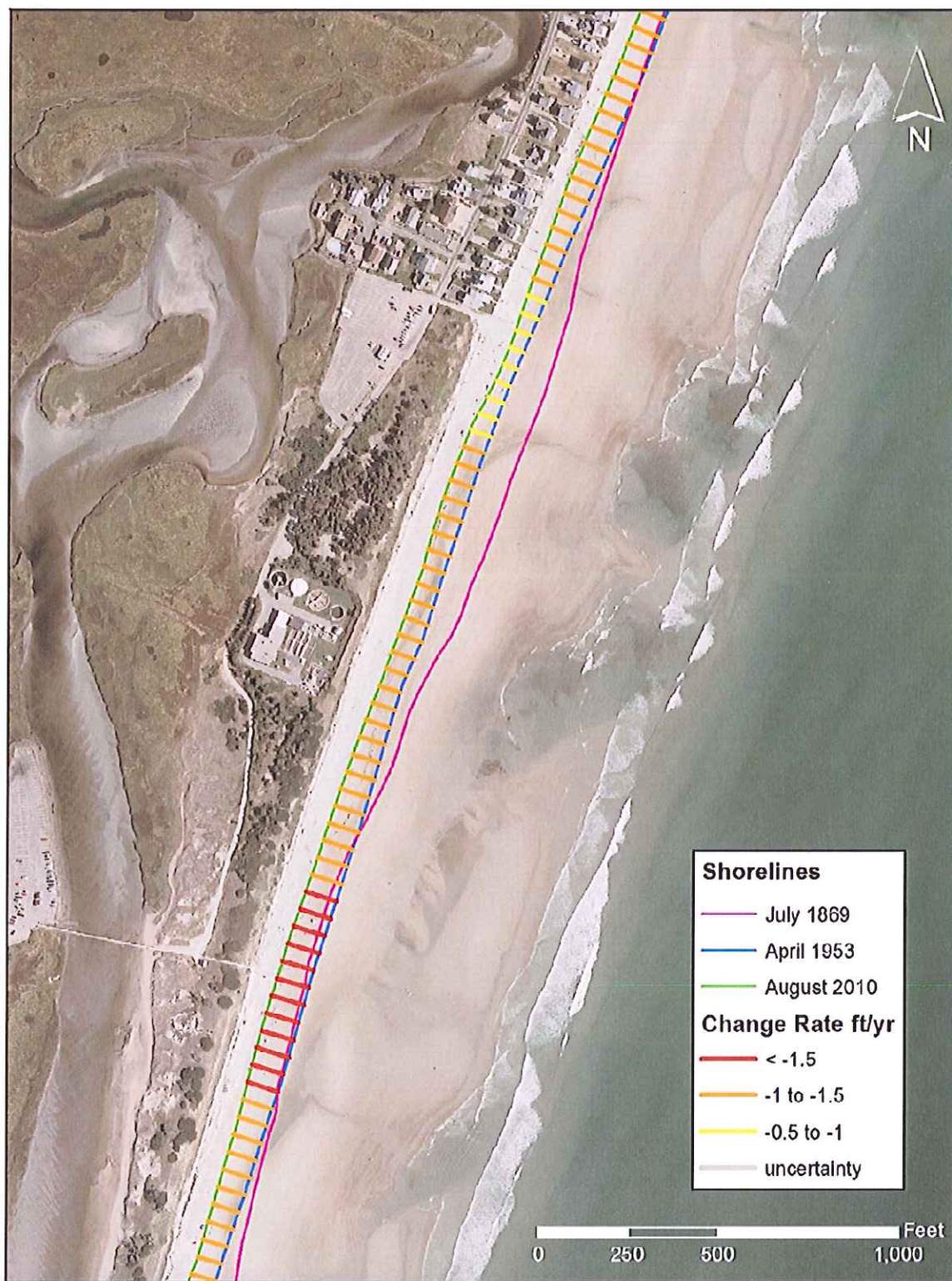
Figure 14. Long-term shoreline change between 1953 and 2010 for the section of Ogunquit Beach fronting the Ogunquit Waste Water Treatment Plant. Shoreline change is color-coded, where the highest erosion rate is represented as red and areas of minimal shoreline change are represented as grey.
