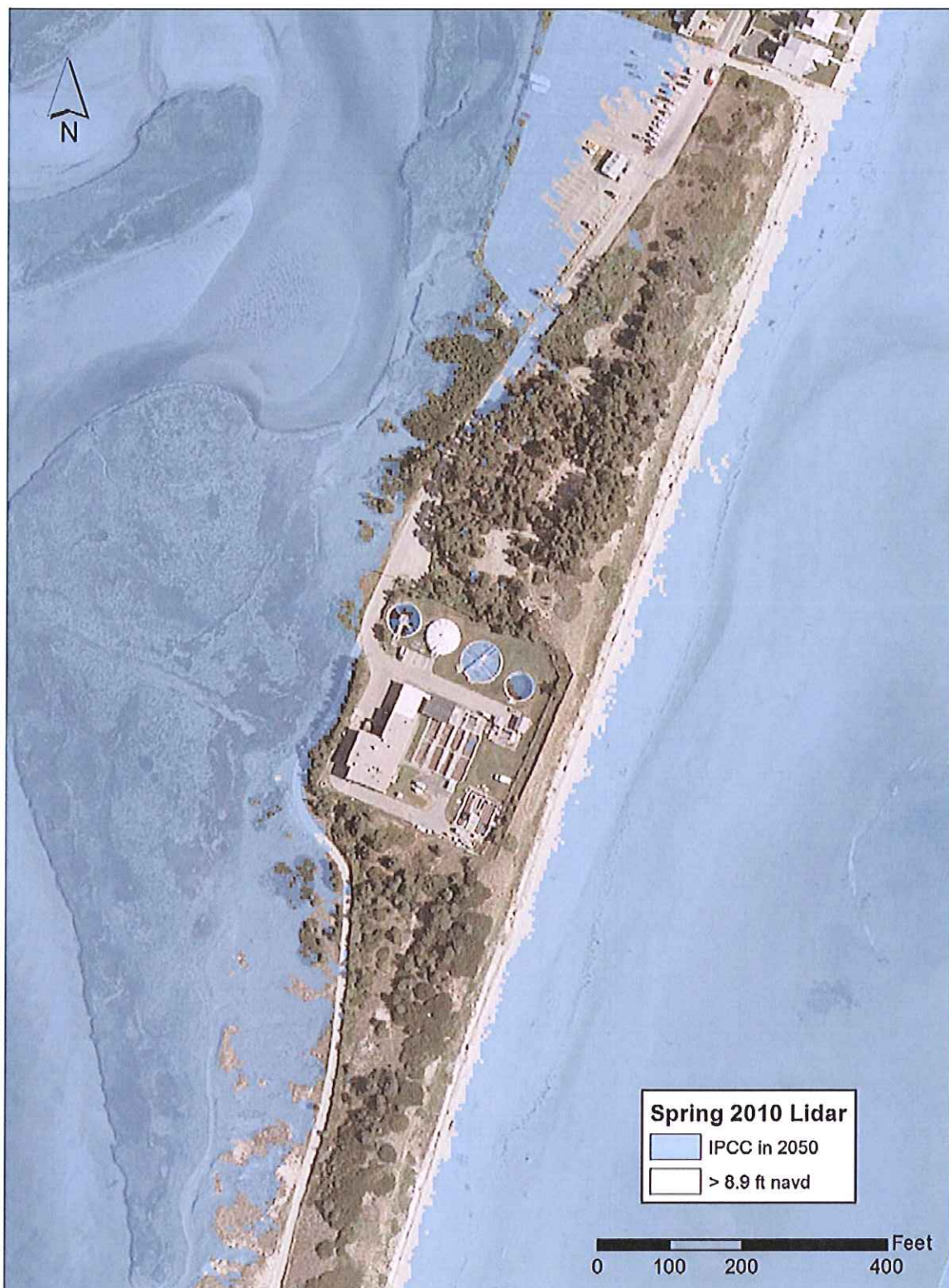
Figure 8. Aerial photograph from 2010 showing the areas that are inundated by flood waters for a 100-year storm event (8.9 feet NAVD) based on IPCC predicted average sea-level rise increase in 2050. The areas shaded in blue would be under water during the storm event. Topographic and bathymetric data utilized for this representation were derived from the 2010 LIDAR survey.
