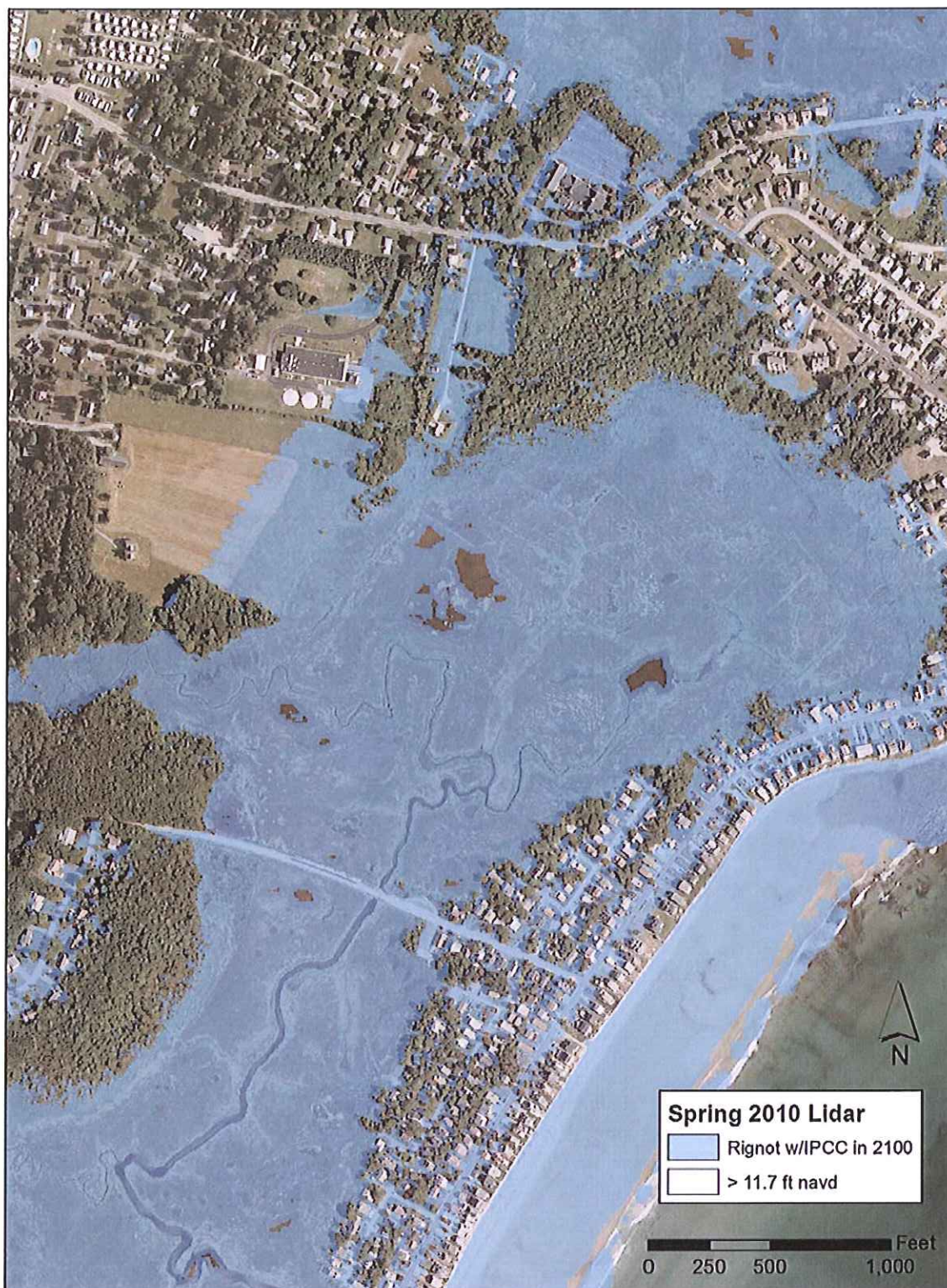
Figure 5. Aerial photograph from 2010 showing the areas that are inundated by flood waters for a 100-year storm event (11.7 feet NAVD) based on IPCC predicted sea-level rise Increase in 2100 including updated input for ice sheet contributions (Rignot, et al. , 2011). The areas shaded in blue would be under water during the storm event. Topographic and bathymetric data utilized for this representation were derived from the 2010 LIDAR survey.
