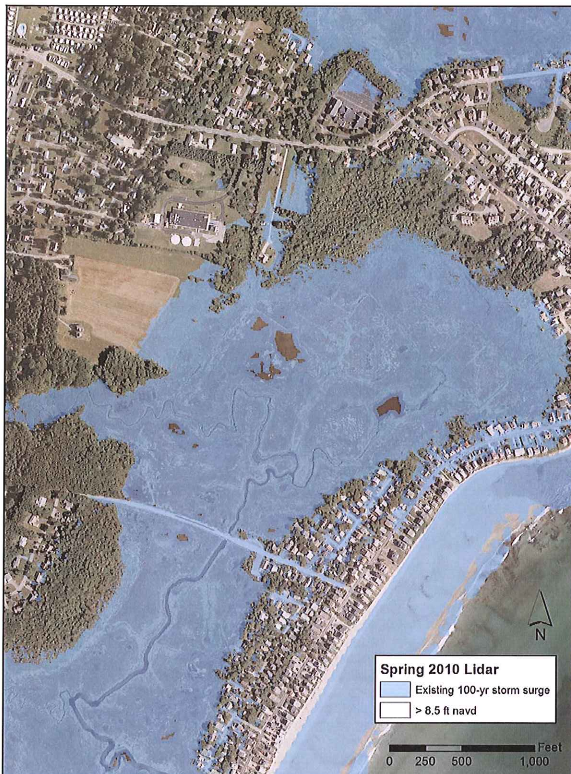
Figure 1. Aerial photograph from 2010 showing the areas that are inundated by flood waters for a 100-year storm event (8.5 feet NAVD) based on existing conditions. The areas shaded in blue would be under water during the storm event. Topographic and bathymetric data utilized for this representation were derived from the 2010 LIDAR survey.
