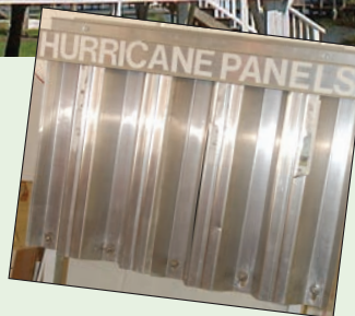
Figures 4-15. These 0.050 gauge aluminum storm panels offer cost effective storm protection. In this example, panels slip into a track above the window and secure onto a bottom track using wingnuts. Source: Roll-a-way/QMI
