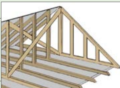
Figure 4-4. Diagonal braces form an X pattern from the top center of the gable end to the bottom center of the fourth truss and from the bottom center of the gable end to the top center of the fourth truss. The same screws as for lateral bracing are used. Source: FEMA's "Against the Wind" brochure 247
